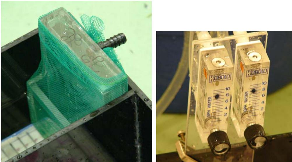
Figure 6 Waterfall box (left) covered in netting to keep salamanders from climbing into it and water flow meters (right).
