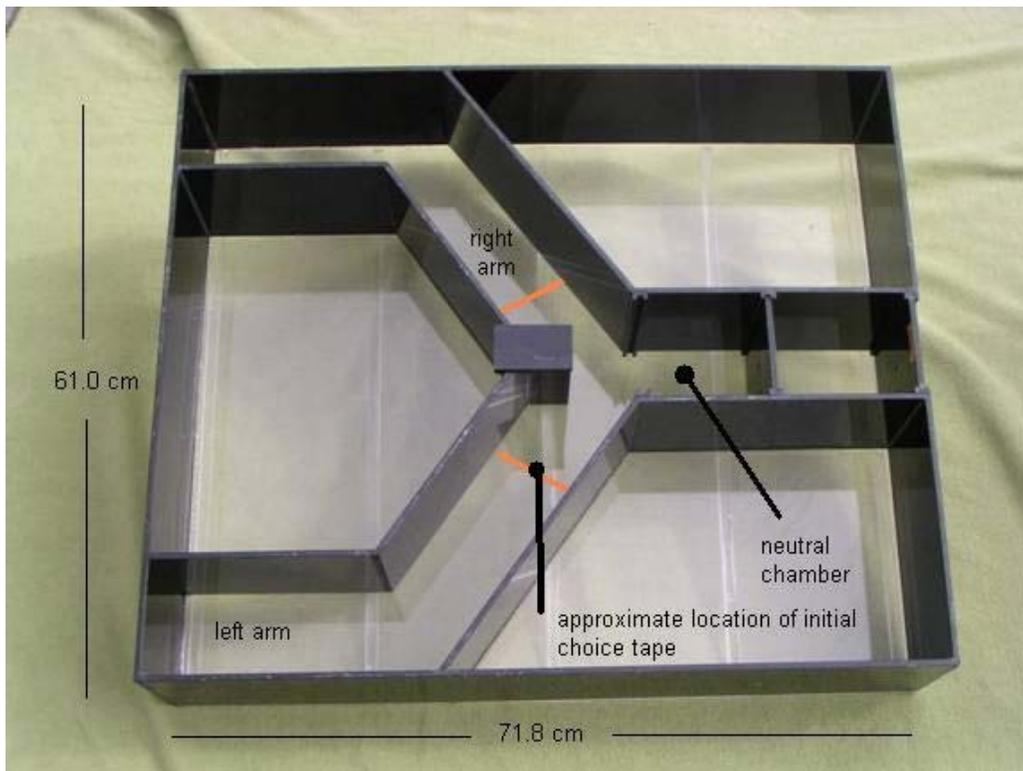
Figure 4 Test station (with door to the neutral chamber removed) used in conditioning and data collecting trials. The chamber to the right of the neutral chamber acted only as a water overflow reservoir. It had no formal function.
